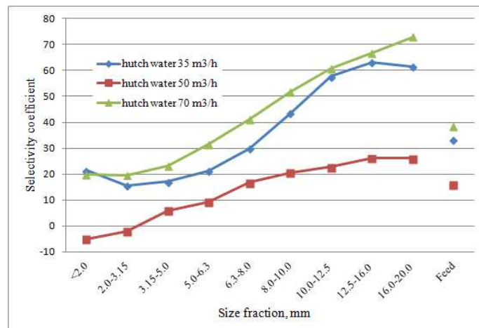
Fig. 5. A change in the value of coefficient f_s obtained under industrial conditions for individual particle size fractions and the feed
