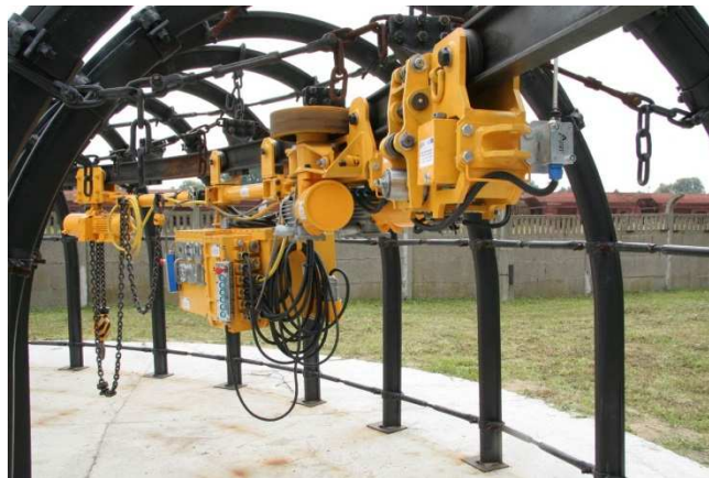
Fig. 4. Suspended battery drivetrain to be used as an example of a machine powered by wireless energy transfer
