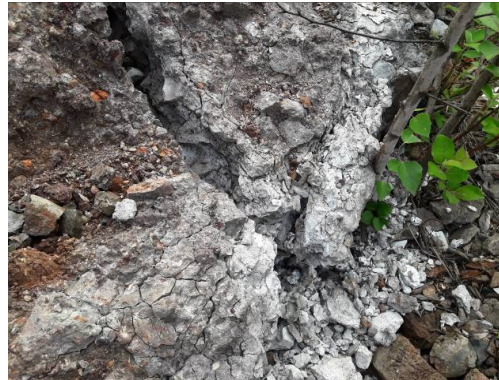
Fig. 4. White bloom of secondary phases
