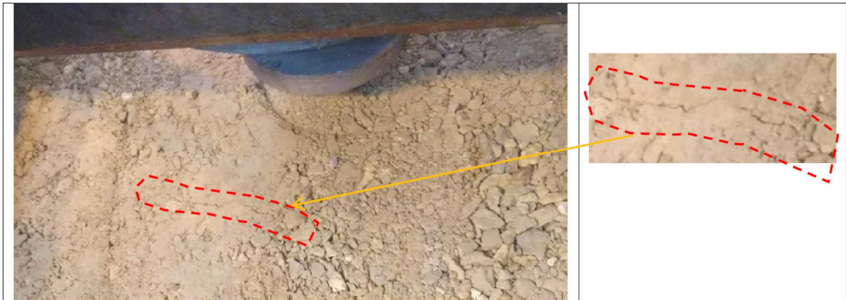
Fig. 16. A new crack on the surface of the aggregate layer after the impact of horizontal tensile strains and the cyclic loading test of 10,000 cycles
