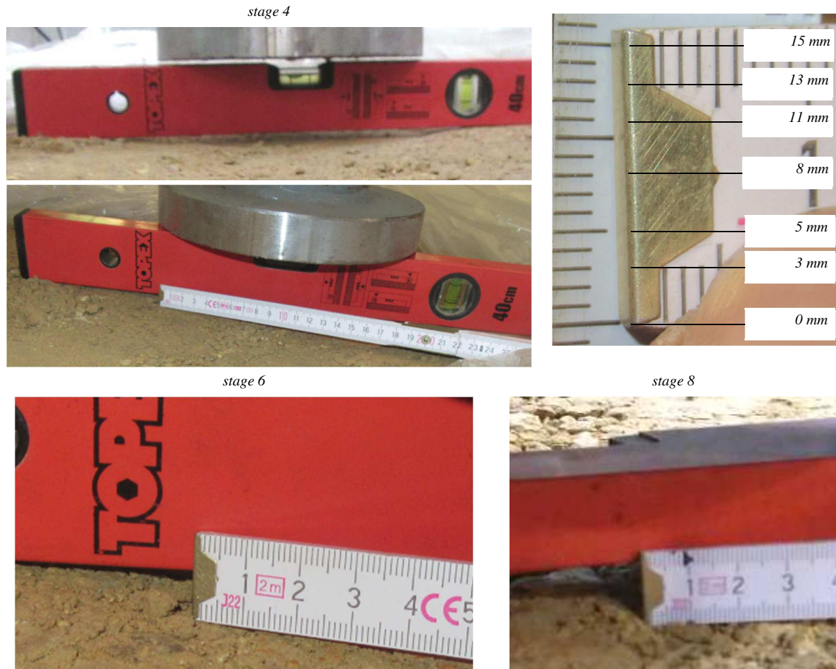
Fig. 18. Subsidence of the pressure plate
