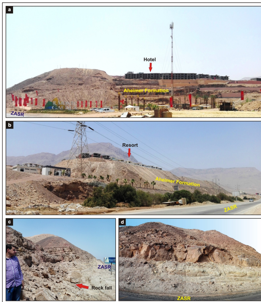
Fig. 2 Field photos of the Paleozoic sandstone facing the Zafarana-Ain Sukhna road (ZASR) show (a, b) hotels and constructions above the sandstones, (c) rockfall at a slope, (d) highly fractured rock face.
