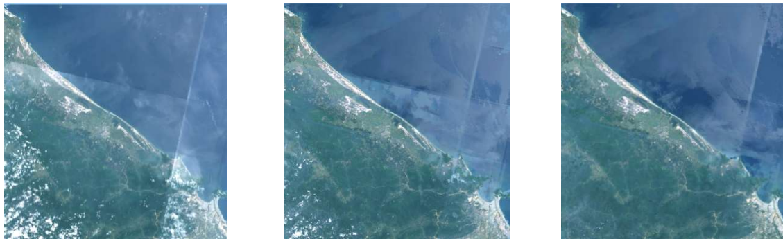
Fig. 4. a. mean composite, b. median composite and c. median composite and clear terrain pixel filtering
