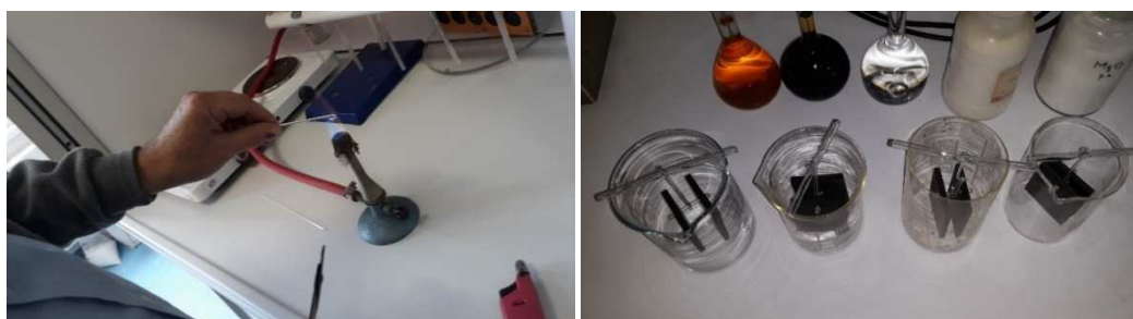
Fig. 3. Creation of hooks (left) and hanging of the samples in the containers (right)
