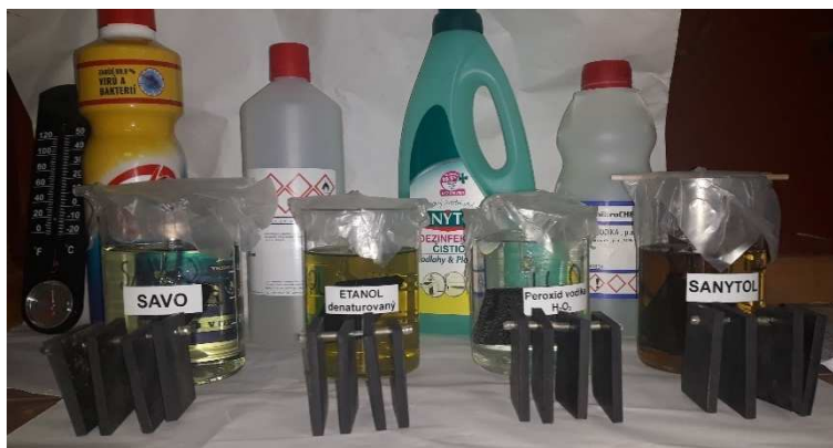
Fig. 4. Prepared samples placed in the containers; from the left: Savo, ethanol, H_2O_2 , and Sanytol
