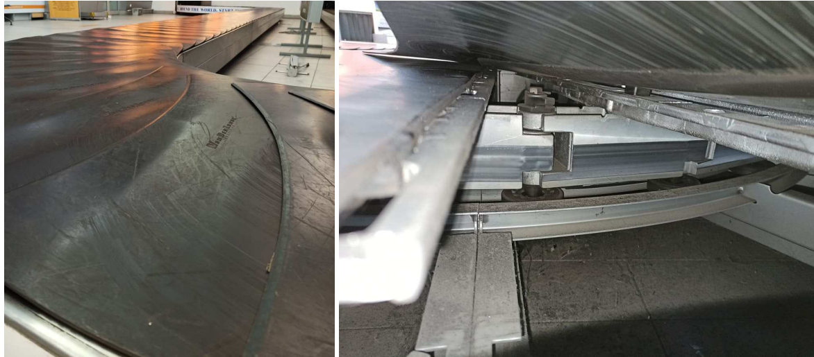
Fig. 11. Baggage belt conveyor in the airport and (on the right) detail of the conveyor under the belt
