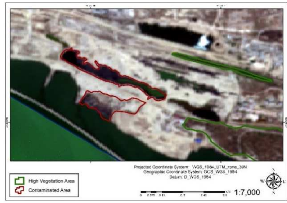
Fig. 8. Sentinel 2, True Color Imagery of the study area. The True Color Image is obtained from Sentinel 2A in the summer season with 10 m spatial resolution. Date: 10.07.2018
