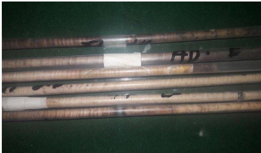
Fig. 3. Storage of Tree ring samples in plastic straw for studying under stereo zoom microscope.
