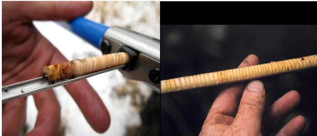
Fig.2. Collection of Tree ring sample using an Increment borer.
