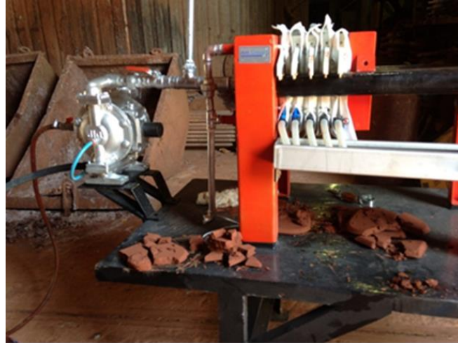
Fig. 3. Laboratory sized press filter.
