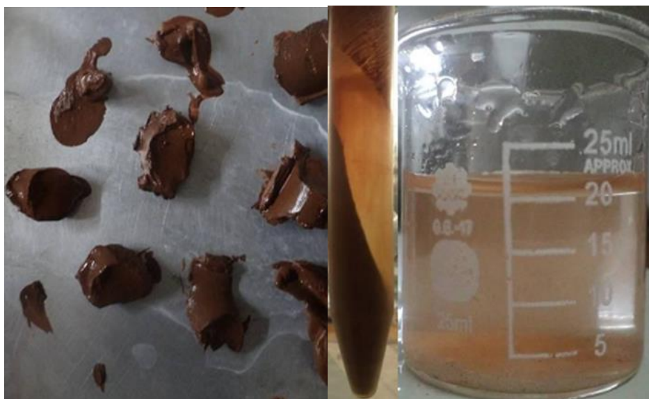
Fig. 12. Centrate and cake image of the sample without flocculant after centrifugation.
