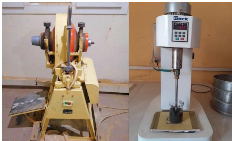
Fig. 4 (a) Laboratory ball mill, (b) Agitation system
