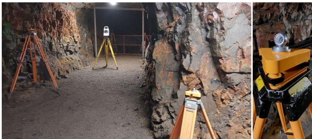
Fig. 4. Josef URC – experimental network, standpoint 6 (left), detail of the reflective prism (right)
