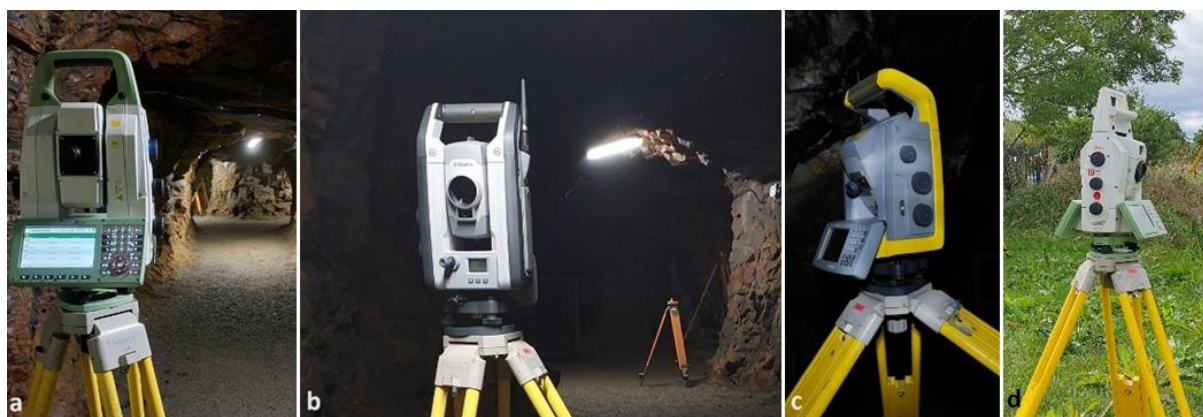
Fig. 1. Total stations tested – a) Leica MS60, b) Trimble S9HP c) Trimble S6HP d) Leica TS60
