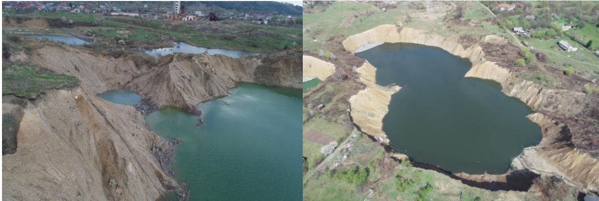
Fig. 3. Left - pictures of some sinkholes in the Solotvyno salt mining area (credit: Ivan Prodanets); right - Flooded mine No. 7 (aerial photography materials as of 2020 carried out using a UAV – Tarot 680PRO Hexacopter)
