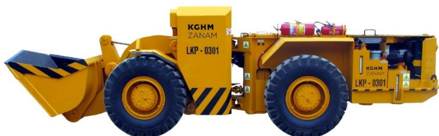
Fig. 2. LKP-0301 loader with the Z-kinematic system, produced by KGHM ZANAM S.A. (KGHM Zanam, 2024)
