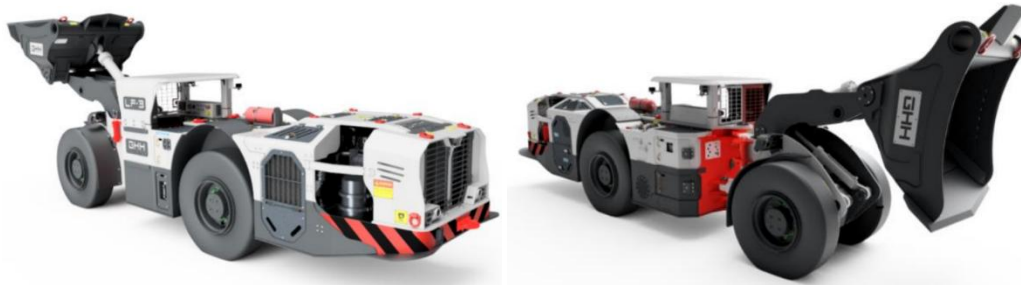
Fig. 3. LF-3 loader with the T-kinematic system, produced by GHH Fahrzeuge GmbH (GHH Fahrzeuge, 2024)
